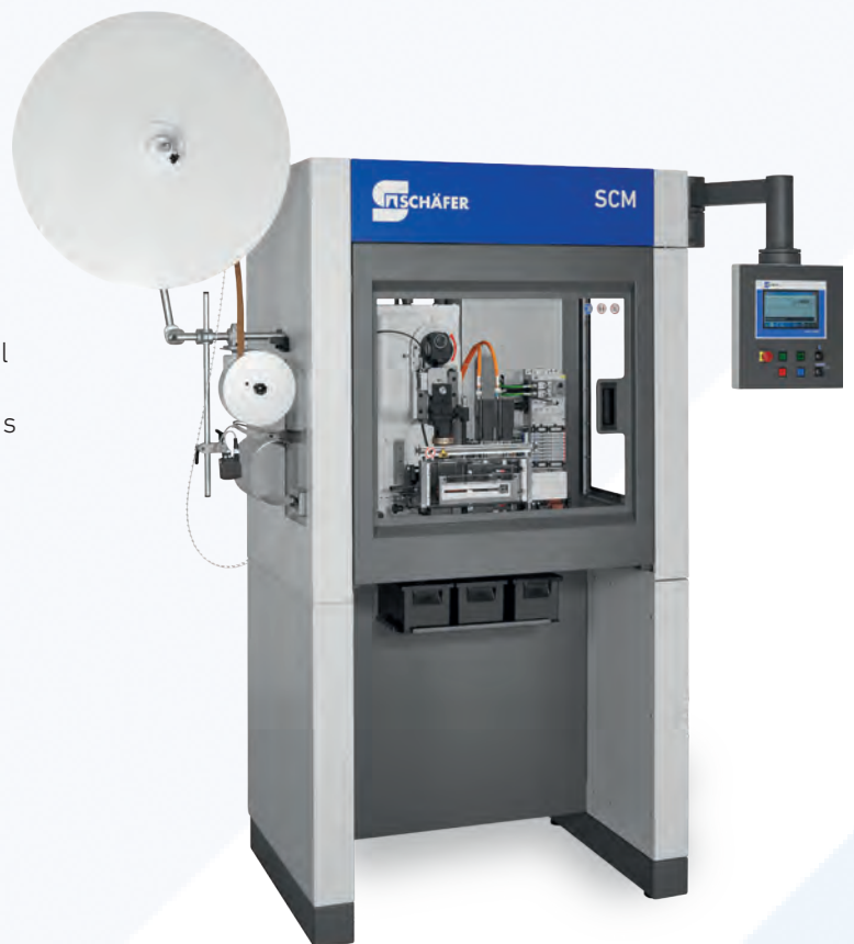
Crimping machine SCM with integrated BB07i4 and SDS100.
